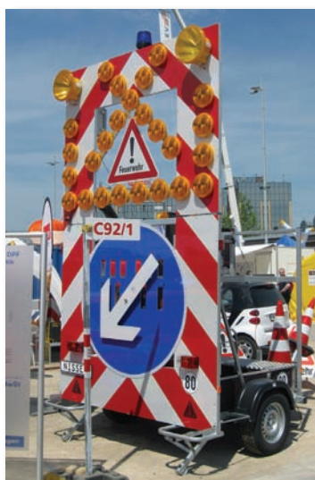
Figure 3.30. This trailer contains a large arrow board.
